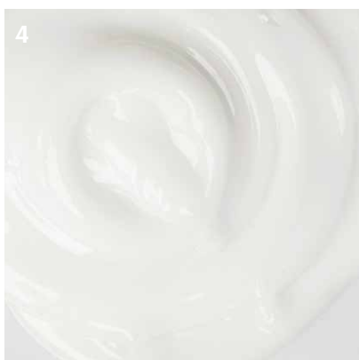
From broken windshields – to laminate fractions – to flakes – to adhesive
