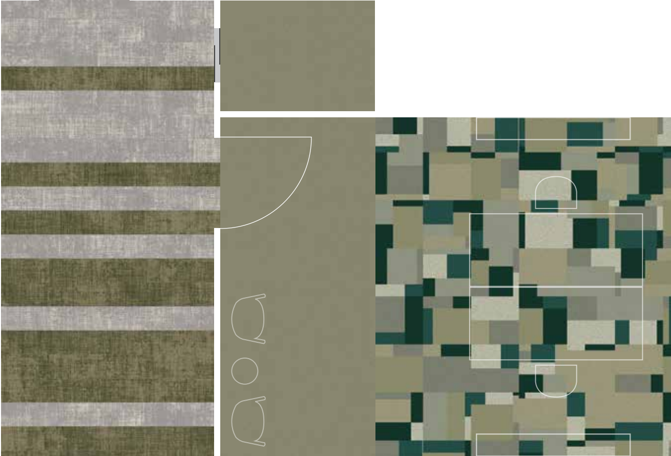
CONFERENCE ROOM: RFM55002105 BORO WEAVE / RFM55202116 MANTRA WEAVE 48x48 CM TILES / CORRIDOR: RFM55002105 / RFM55952128 BORO WEAVE 24x96 CM PLANKS / LIFT: RFM55202115 SHADE 48x48 CM TILES / OFFICE: RFM55202115 SHADE / RFM55202110 BLOCK SHADE 48x48 CM TILES
